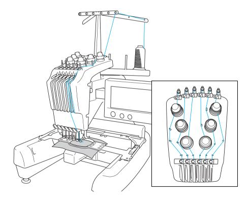
The numbers indicate the thread path for each of the numbered needle bars. Be very careful to correctly thread the needle bars.
